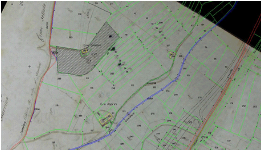
Figure 2 - Digitization of a raster map
