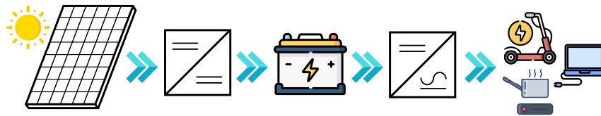
Fig. 3.9 Typical power conversion chain of an off-grid PV-storage system supplying local DC or AC loads.
