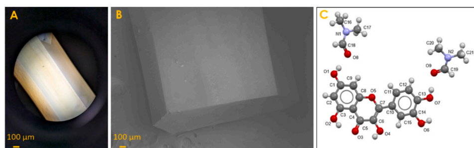
Fig. 2. Micrograph (A), SEM image (B), and chemical structure of QDMF crystals (C).
