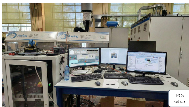
Fig. 5.3 View of the real-time control PCs setup.
