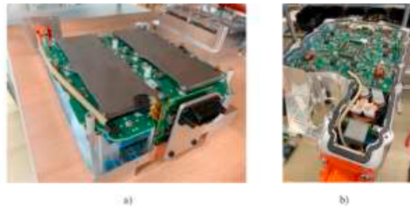
Fig. 4. a) Prototype inverter with power stage on top and cooling fixture below; b) prototype inverter in integrated inverter-e-motor housing.
