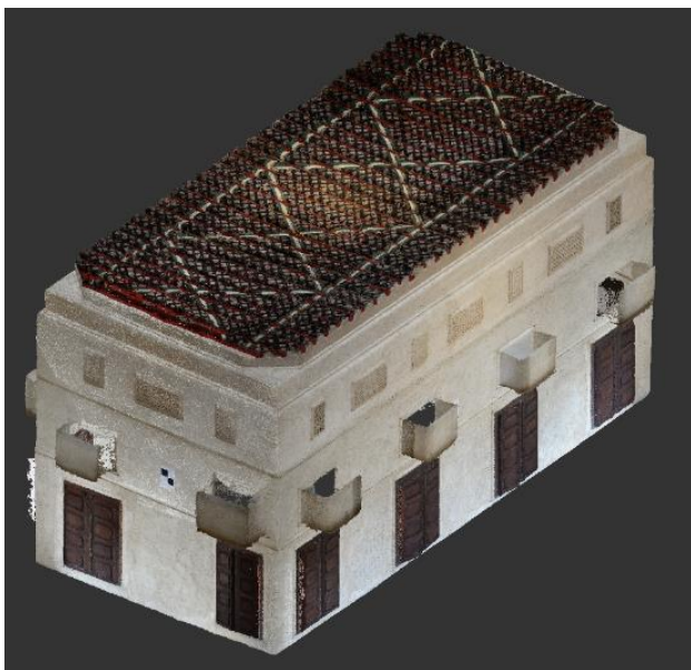
Figure 5 Point cloud of a room entirely generated from photogrammetry.
