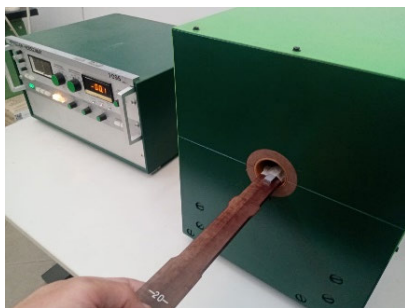
FIGURE 5. Specimen insertion in the coercimeter coil.
