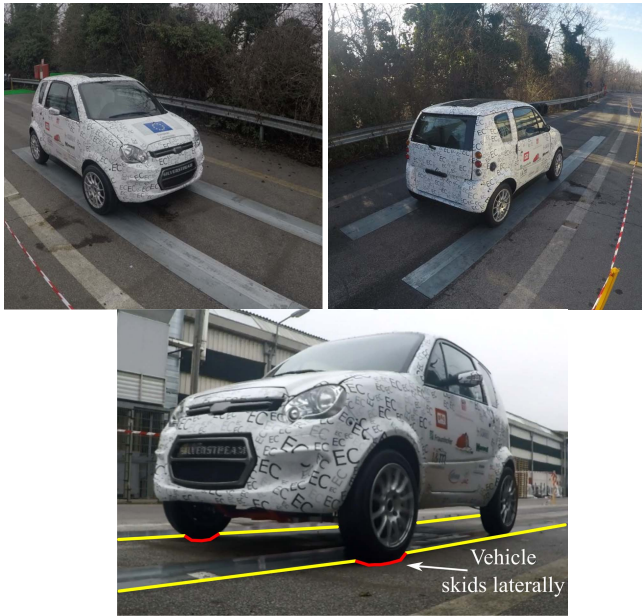
Fig. 13. Electric vehicle prototype during the TC and passive vehicle experimental test session on the low- \mu metal plates. The vehicle skids laterally when the TC is deactivated (bottom).
