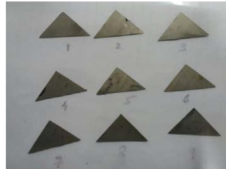
Fig. 1. Machined Titanium alloy specimens
