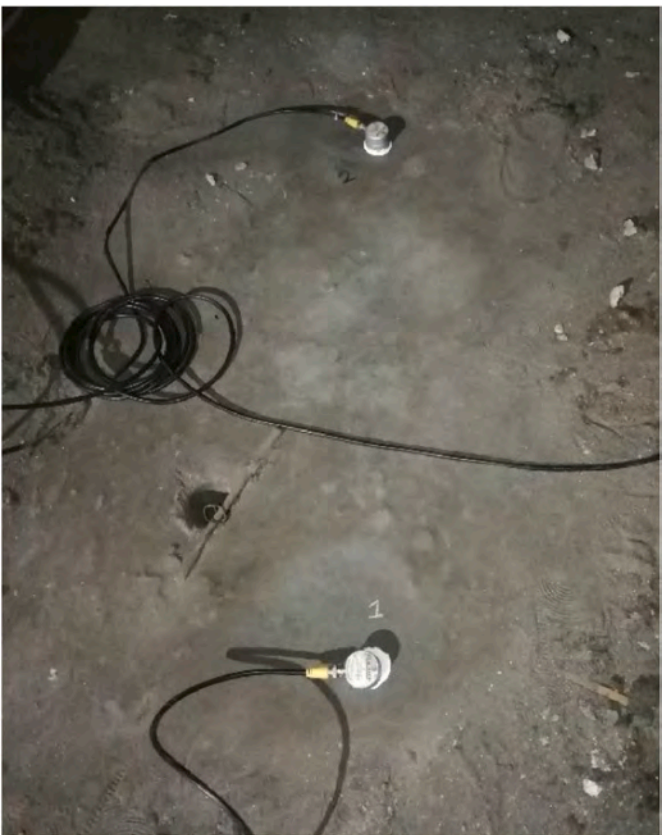
Fig. 7. Two of the eight sensors, positioned on the extrados of the central nave vault.
