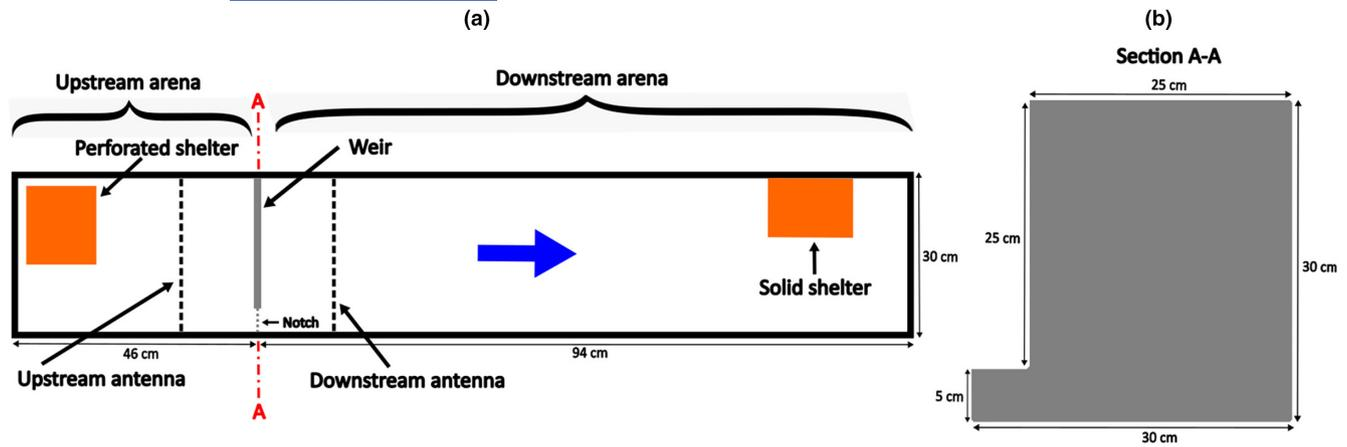
**FIGURE 1** A scaled drawing of the experimental arena: (a) top view of the experimental arena inside the flume (the blue arrow indicates the flow direction), (b) front view (section A-A) of the deep side notch weir. The upstream end of the flume is delimited by a flow straightener, and the downstream end by a fine-meshed rack.
