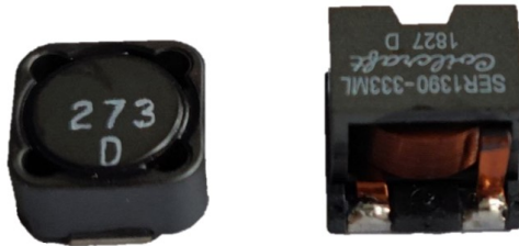
Fig. 3.3 Photo of the two tested inductors. The MSS1260T-273 is on the left, the SER1390-333 is on the right.
