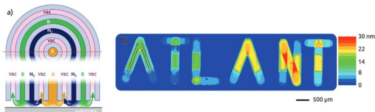
Fig. 1: a) Microfluidic precursor delivery concept: schematic view of the delivery nozzle in frontal view (top) and in cross-section (lower panel). b) Demonstration of direct pattern generation: Pt-printed ATLANT logo featuring letters from A to T obtained with 140, 150, 170, 190, 200 and 210 individual passes, respectively [1].
