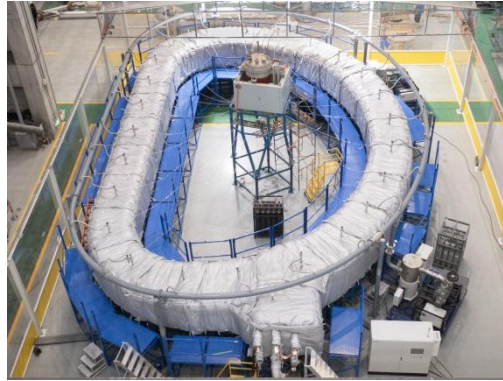
Fig. 1: Vacuum pressure impregnation for the TF WP.
