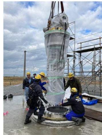
Fig. 1: Liquid hydrogen circulation test of an HTS submerged pump at JAXA Noshiro Rocket Facility (Japan) [3].
