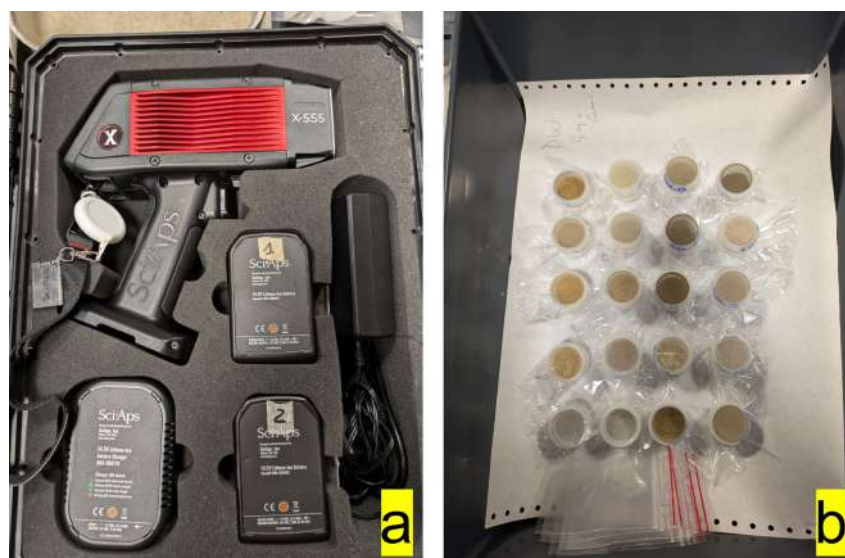
Fig. 4.13 (a) Portable pXRF instrument used for geochemical screening, a SciAps X-555 handheld X-ray fluorescence spectrometer operating up to 55 kV. (b) Powdered samples prepared for pXRF analysis, placed in plastic sample cups and sealed with thin film.
