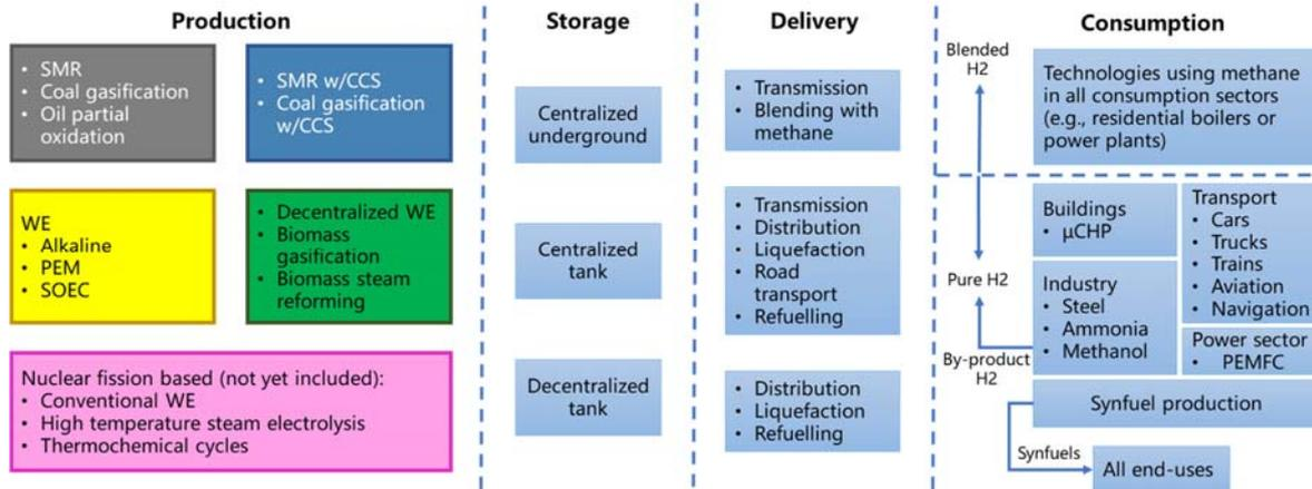
Fig. 1 High level representation of hydrogen value-chain, distinguishing among different qualities of H<sub>2</sub> based on the typology of production [15]
