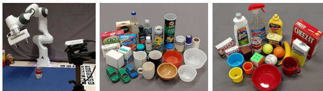
Fig. 6. Left: Our real experiments setup with Franka Panda robot and Realsense D415. Center: Custom set with 28 objects from similar categories as in ShapeNetSem-8 (from left to right and top to bottom: 6 boxes, 5 bottles, 2 soda cans, 5 cylinders, 3 toy cars, 3 mugs, 4 bowls). Right: Selection of 20 YCB objects including shapes from unseen categories.
