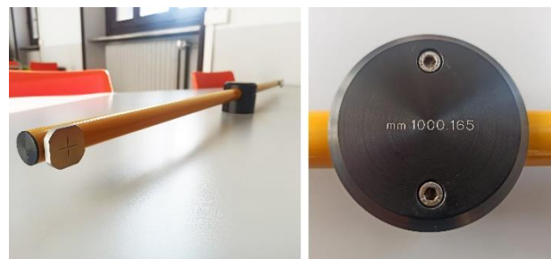
Figure 7. Calibrated Invar metric bar.
