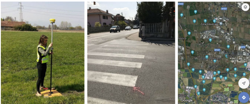
Fig. 12.2 GCPs materialized in the surveyed area and GNSS receiver (a). Natural point selected as GCP (b). Overall view of the GCPs (c). (Images from the 3D metric survey carried out by the Geomatics group of Politecnico di Torino)
