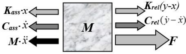
Figure 2 Schematic representation of the force equilibrium along the x-axis.
