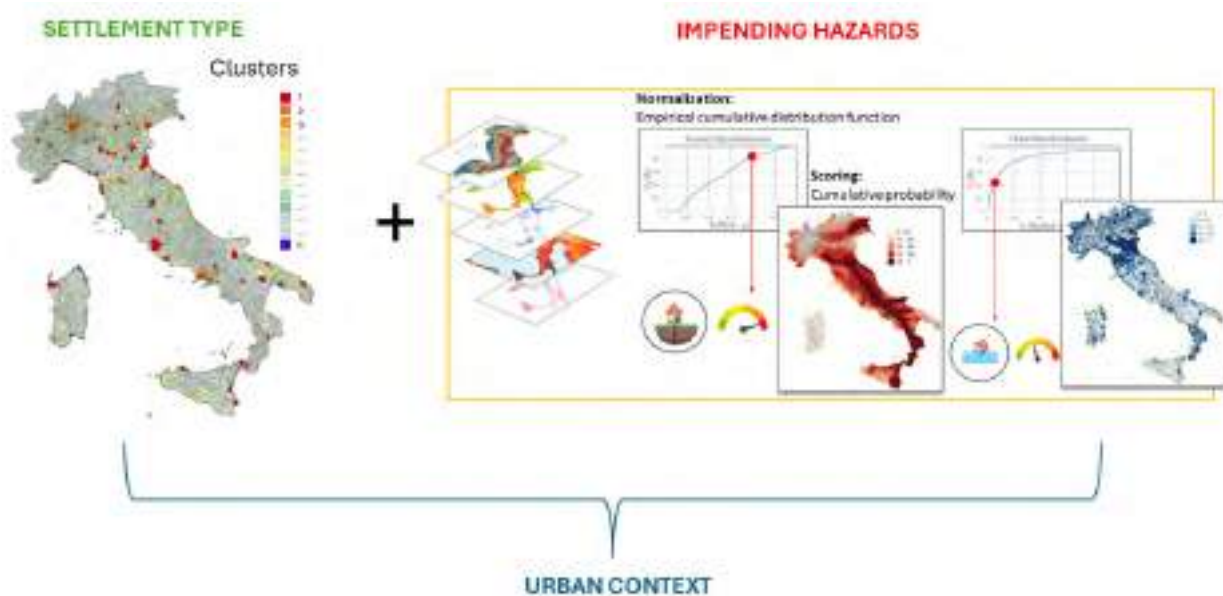
Figure 1 –Urban context is defined by the settlement type and the impending hazards. An example of score-based procedure for the identification of relevant hazards is reported, comparing seismic and flood hazards.
