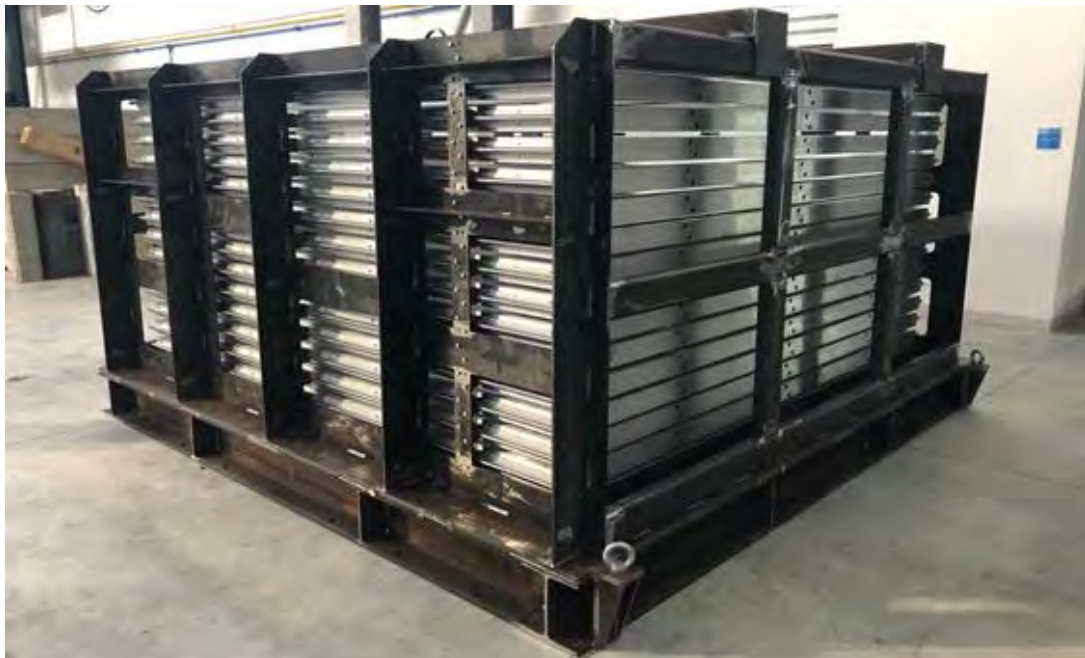
Figure 1 - Laminar shear box at the Laboratory of Earthquake engineering and Dynamic Analysis (L.E.D.A.).
