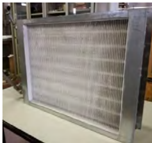
Figure 4. Picture of the SAPO-34 ADS-HX
