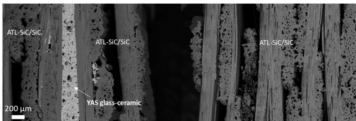
Fig. 12. FE-SEM cross-section of fracture surfaces of YAS glass-ceramic ATL-SiC/SiC flat-joint, obtained with joining process P2, after performing SLO shear tests. The failure was caused by the delamination of the CMC.
