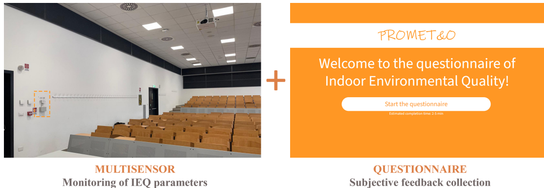
Figure 2: Multi-sensor flush to the wall in classroom 4P (left) and homescreen of the PROMET&O questionnaire webpage (right).
