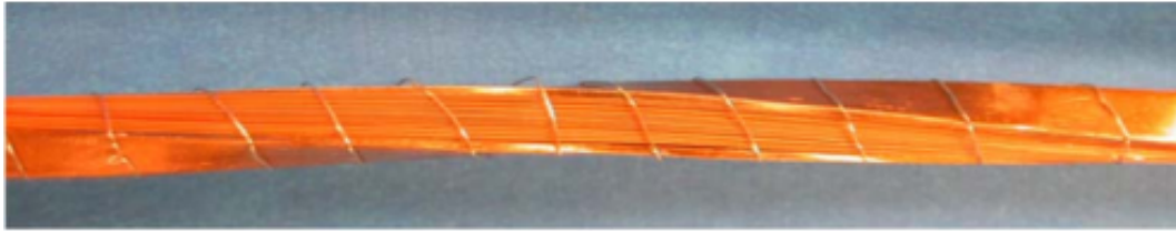
Fig. 1.5 Picture of twisted stack of ReBCO tapes. ©2013 IEEE. Reprinted, with permission, from [26].
