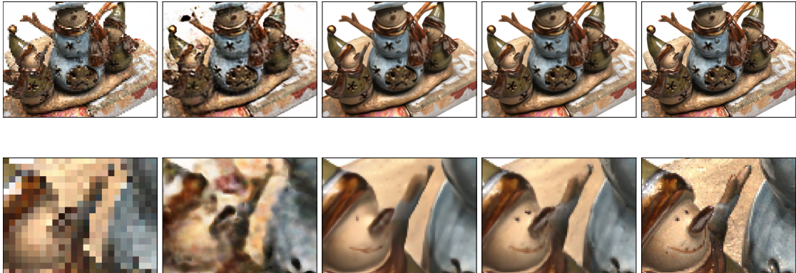
Figure 3.2: DTU scene 3 with 4\times scale factor. From left to right: LR nearest neighbours interpolation (19.31 dB), NeRF-SR (19.75 dB), BSRT (23.60 dB), EpiMISR (24.43 dB), HR ground truth.
