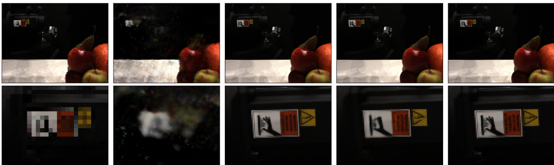
Figure 3.6: A qualitative example of a failure case (DTU dataset, scan 63). This is an example where BSRT outperforms EpiMISR. From left to right: LR nearest neighbours interpolation, NeRF-SR, BSRT, EpiMISR, HR ground truth.
