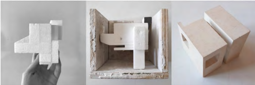
Fig. 3. Styrofoam negative, 10cm mold, a 10cm cube with cast interior of a room inside.
