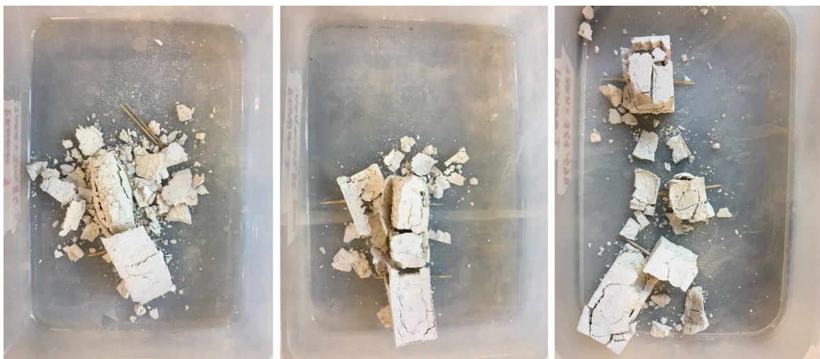
Figure 12. Tested samples of two-component grout after one month of curing.
