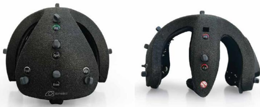
Figure 2: Wearable and portable electroencephalograph by ab medica.
