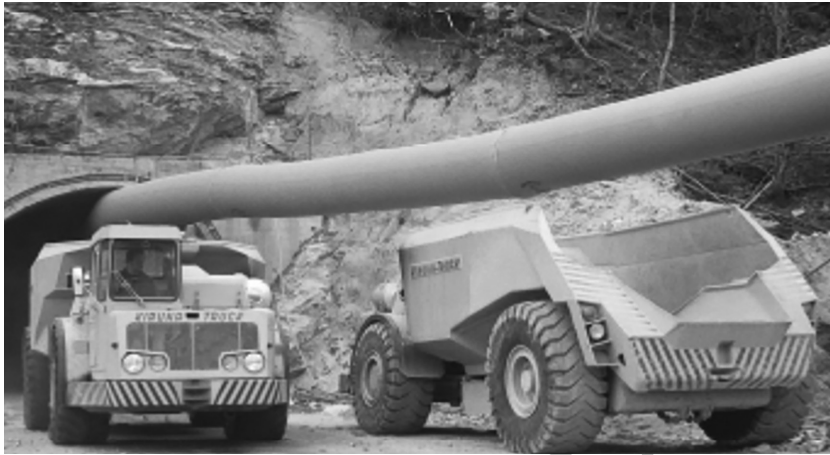
Figure 6.14 Kiruna Truck K350.
