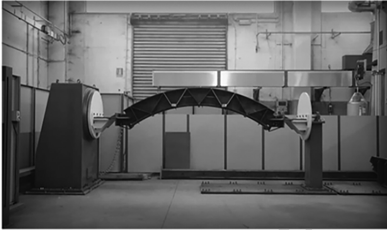
Figure 6.37 Example of robotized alternate side shutter welding process to distribute tension effects.
