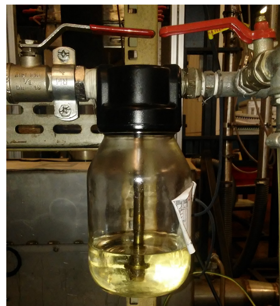
Figure 3. Synthetic (DEHS) aerosol generator.
