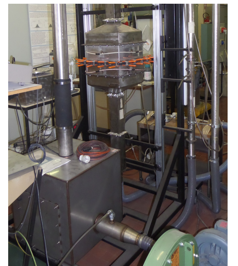
Figure 4. Filter media test rig.
