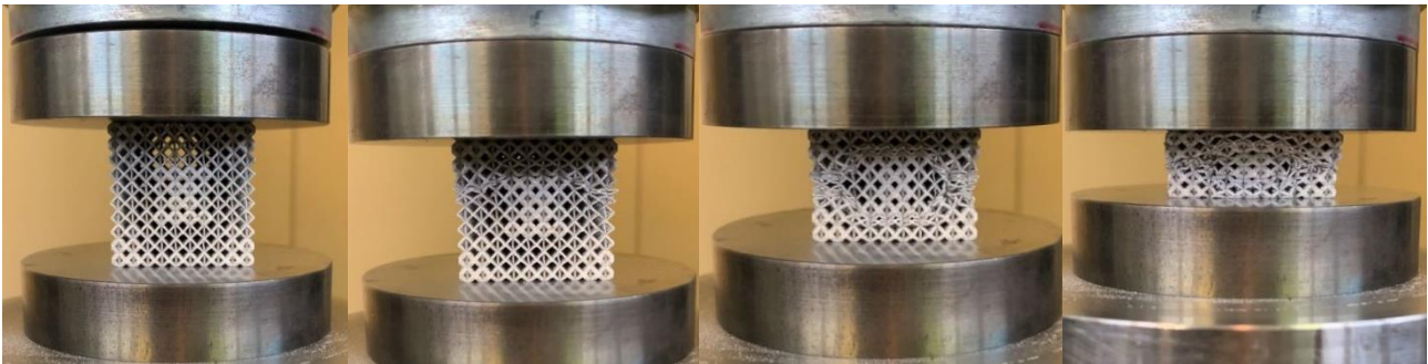
Figure 2: compression test of the bccz sample graded using process P1
