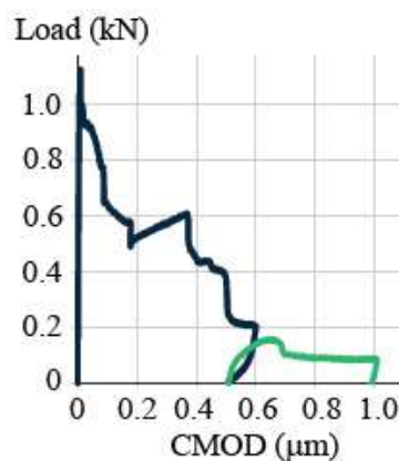
Fig. 7. Example of a load vs CMOD curve resulting from pre-loading (black curve) and re-loading (green curve) stages for a sample with a coated capsule.
