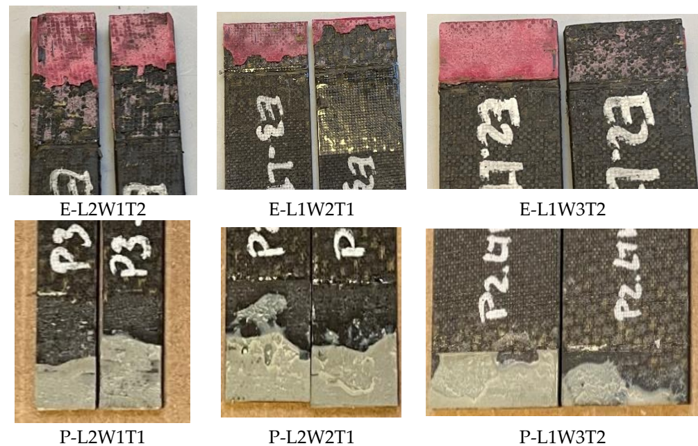
Figure 13. Failure surfaces of the specimens after the test.
