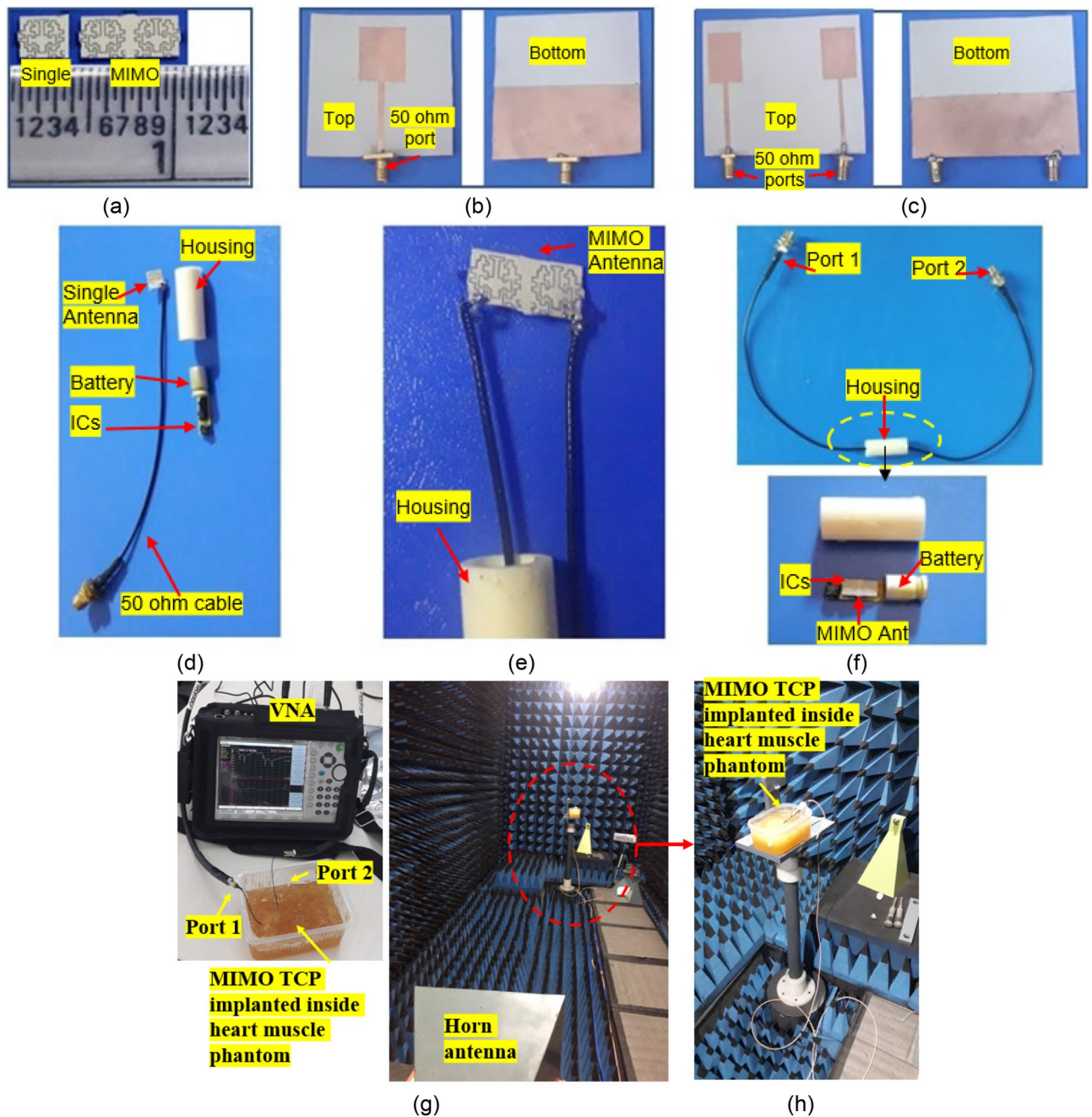
Figure 5. Fabricated prototypes and measurement set-ups. (a) Fabricated prototypes of single and two-port MIMO implantable antennas. (b) Single-port outside body antenna. (c) Two-port outside body MIMO antenna. (d) Single-port TCP capsule with antenna and electronics. (e) Single-port TCP capsule with antenna and electronics. (f) Two-port MIMO antenna with TCP housing. (g) Near-field measurement of implantable MIMO antenna. (h) far-field measurement of implantable MIMO antenna.
