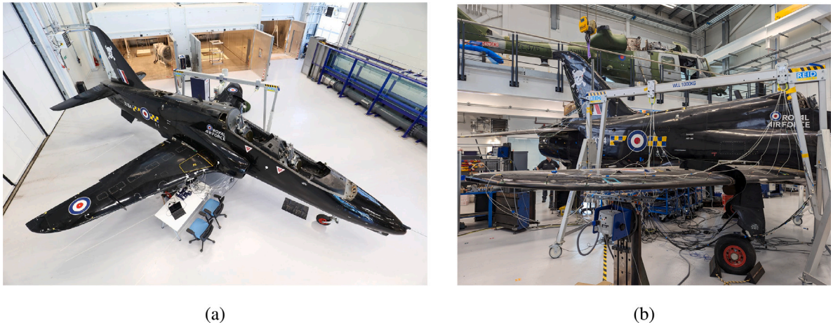
Fig. 6. Hawk T1A Aircraft: first (Fig. 6(a) – retrieved from Haywood-Alexander et al. (2024)) and second test setup (Fig. 6(b) – retrieved from Wilson et al. (2024a)).
