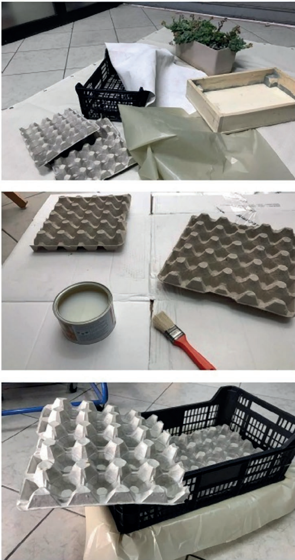
Figure 21 | Blue-Green Roof Module prototype with recycled materials. Source: Dadati & D’Amico, 2020, p.147.
