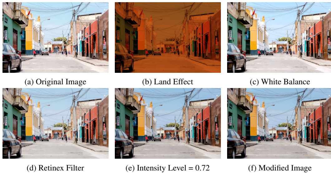
Fig. 2.23 Experimental results for a sample image named B07.png. The modified image (f) consumes 19.75% less power than the original image (a) and is preferred by 71% of the participants of the subjective test.
