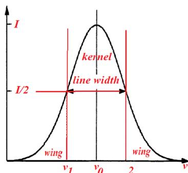
Fig. 3: Kernel and wings (tails) of a line.
