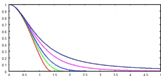
Fig.4: q- exponential functions in the case of  $\gamma=2$  (blue,  $q=2$ , Lorentzian; pink  $q=1.5$ ; light blue,  $q= 1,01$  near Gaussian; green,  $q=0.75$ ; red,  $q=0.5$ ) For  $q < 1$ , the function is different from zero in a limited interval. Being the line symmetric, only the right part of it is given in the figure. The same we will do in the following figures.
