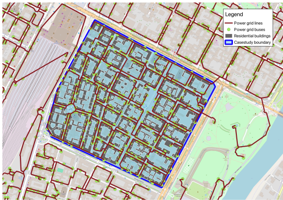
Fig. 5. QGIS visualization of the generated output of CIM Wizard for the case study
