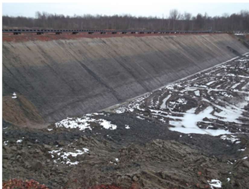
Figure 3. Clay layer at the overburden: the material is exploited for brick production (credits C. Oggeri).
