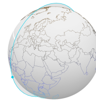
FIGURE 11. Earth observation mission in a 500-km altitude sun-synchronous orbit.
