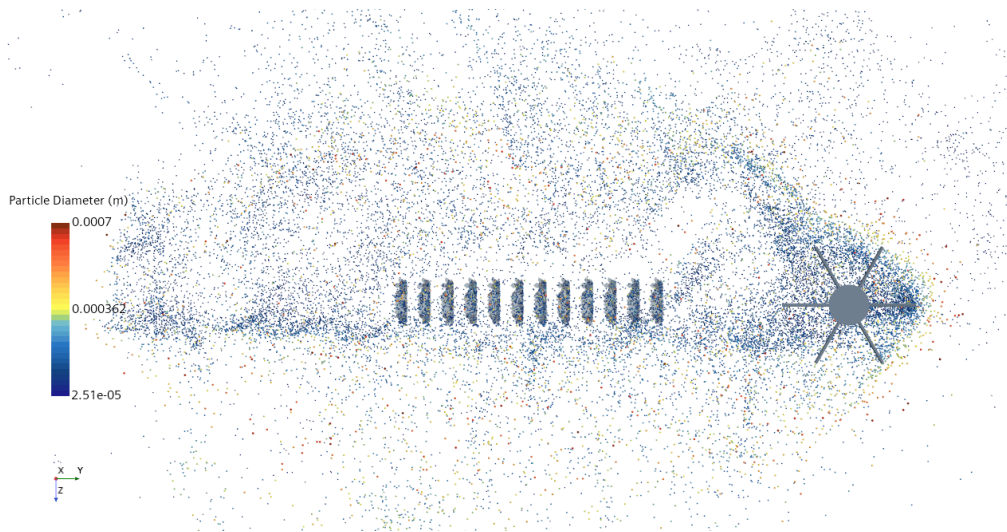
Fig. 8.30 Top view of droplet distribution with 80^\circ hollow cone nozzle (Real cone angle set to 56^\circ ). T=4.0 s.
