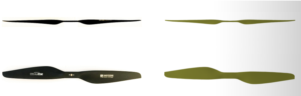
Fig. 4.3 Comparison of top and front views of the original (left) and digitally reconstructed (right) blade.
