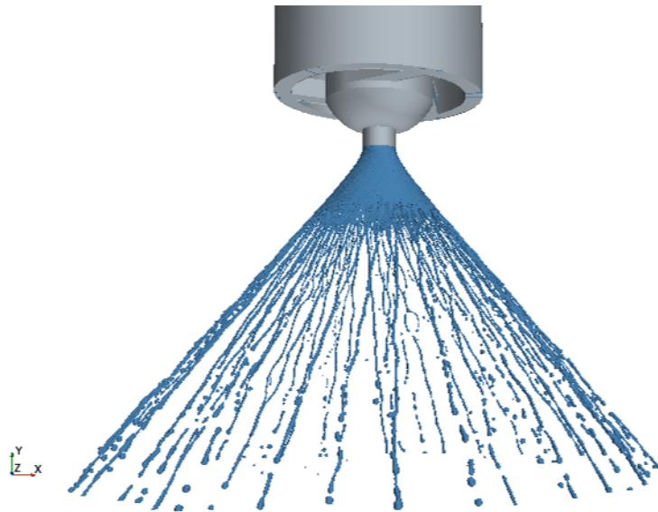
Fig. 8.16 Water-air interphase in VOF CFD simulation showing the conical sheet of fluid produced by the pressure swirl nozzle at a pressure of 2 bar.
