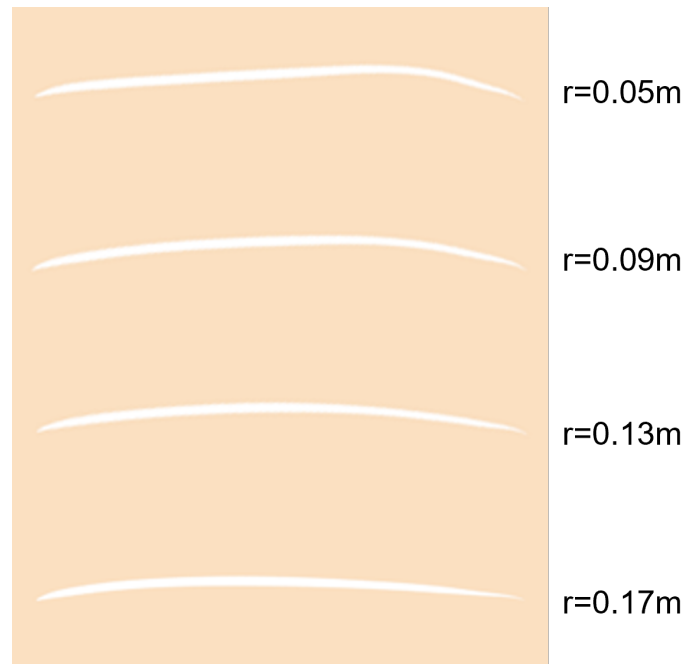
Fig. 5.15 Normalized airfoil sections at different radial stations after adjoint optimization. Two-bladed rotor.
