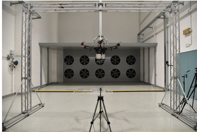
Fig. 8.1 UASS and Camera Setup in the SEASTAR Wind Tunnel.
