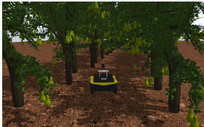
Fig. 1. The proposed SegMin and SegMinD algorithms allow to precisely guide an autonomous mobile robot through a dense tree row solely using an RGB-D camera. A pear crop row in Gazebo is shown in the picture.
