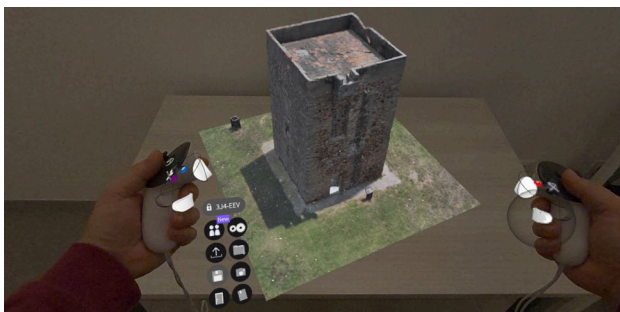
Figure 6. The MR environment using Gravity Sketch enables multi-scalar inspection and 3D annotation directly on the model. (Prototyping: E. Pupi)
