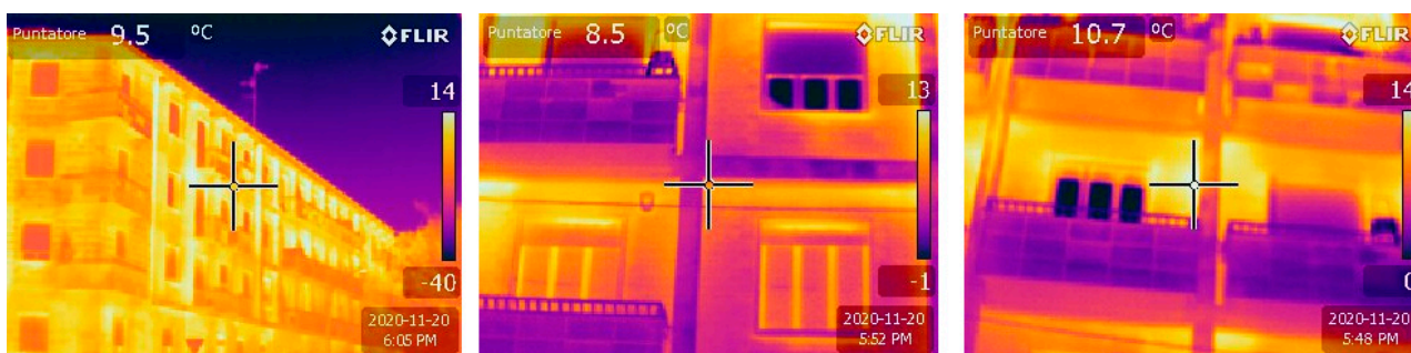
Figure 7. Thermographic analysis of the building envelope. Images taken by the authors.
