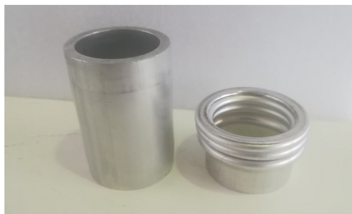
Figure 2: Aluminum specimen for impact energy absorption evaluation and deformed shape after compression test.
