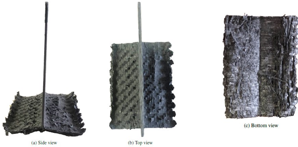
Figure 24: Splaying failure mode found on GG630T-37 carbon/epoxy specimens after crashworthiness test [96].
