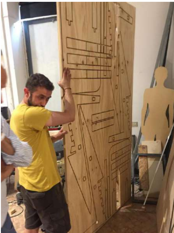
Fig. 12: A young designer, operator at Science City Foundation of Naples Fab Lab holds the plywood sheet with the layout of “Fit It!” chairs in their 2.0 version.
