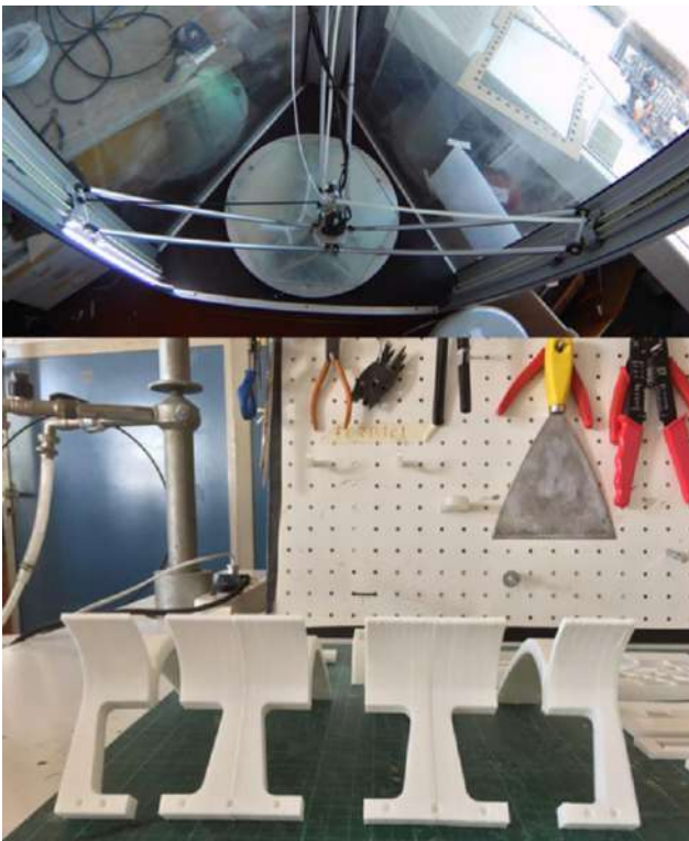
Fig. 10: Realisation of the scale model of the dwelling unit at +LAB (3D Printing Lab of Politecnico di Milano, arch. Michele Tonizzo). The 3D printing using a polar 3D printer (max. cylindrical printing volume 40 cm x 70 cm) and the extrusion of white PLA filament. Below: post-production of the component modules of roof.
