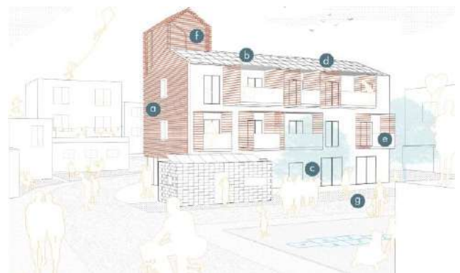
Fig.12: Design strategies. a. ventilated façade; b. photovoltaic modules; c. air to water heat pump; d. solar modules; e. shading system; f. solar chimney; g. rainwater reuse.
