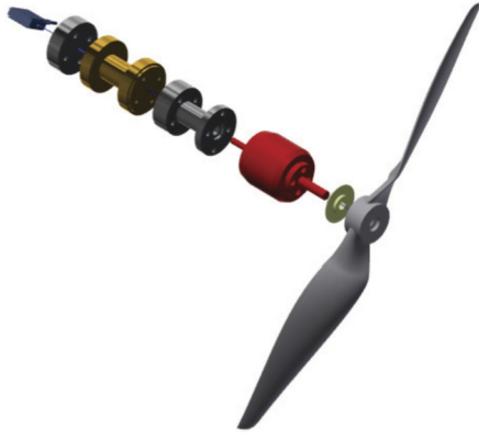
Fig. 2. Exploded view of the propeller drivetrain.
