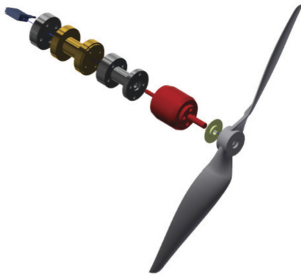
Fig. 2. Exploded view of the propeller drivetrain.
