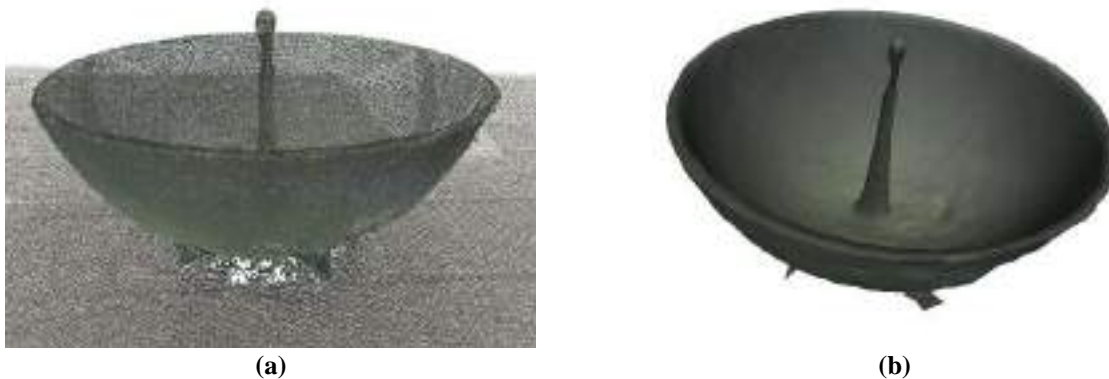
Figure 5 Final points cloud (a) and reconstructed mesh (b).
