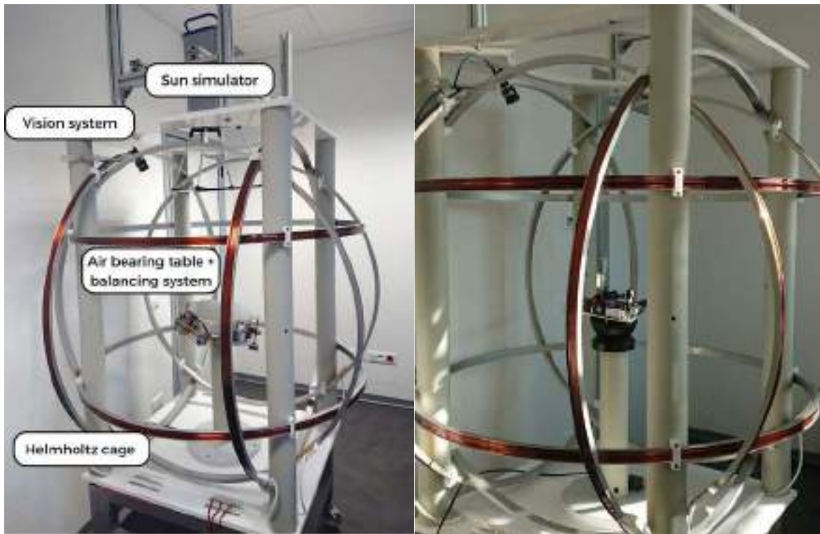
Figure 1: The attitude simulator testbed of the Unibo. The air bearing table for satellites with mass up to 4 kg is shown on the left, the one for satellites with mass up to 1 kg is shown on the right.
