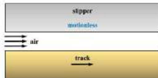
Fig. 1. Gap between slipper and track
