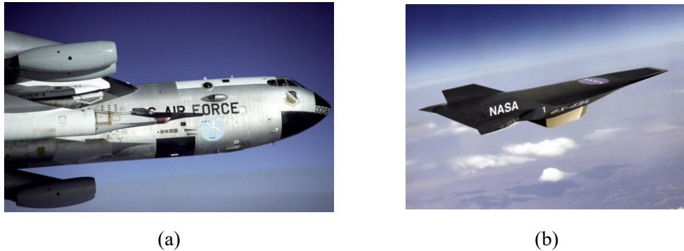
Figure 4: (a) X-43 flight testing through modified Pegasus booster carried aloft by the NASA NB-52B (Credits: NASA Photo (NASA, 2009)); (b) X-43 vehicle after release (Credits: NASA Photo (NASA, 2009))
